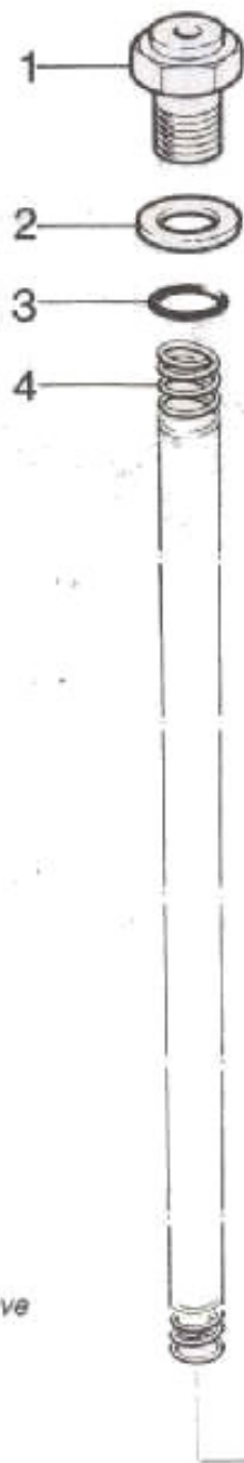
8.10 Exploded view of a typical later model fork leg
